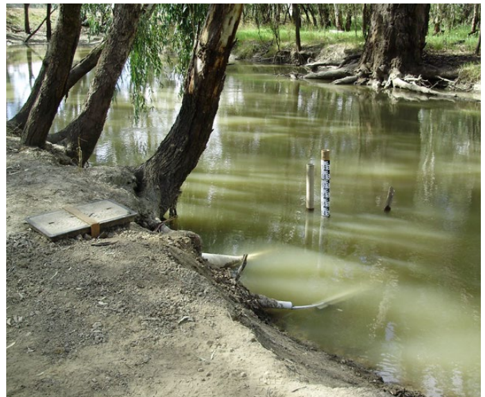
Like the vast network of braided creeks winding through the nearly flat Murray Darling Basin, Colombo Creek in rural New South Wales is highly subject to backwater effects from confluences, trees and other debris, and algal blooms. As a result, gaugings are typically scattered around the rating curve.
