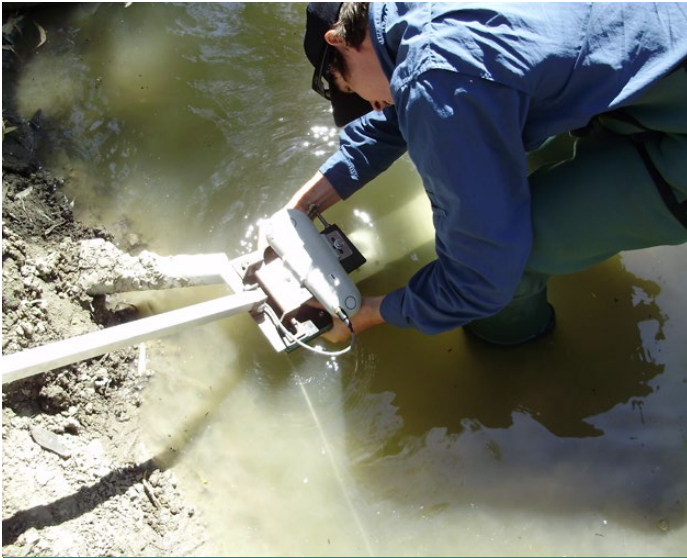
Right out of the box, with just a quick survey of the riverbed and banks input into its onboard software, this SonTek-IQ shallow water flow meter delivered extremely accurate level and flow data.
