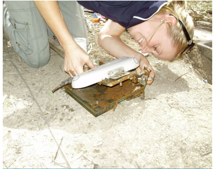
Hydrographer Sophie Gatacre of the NSW Office of Water readies a SonTek-IQ shallow water flow meter for long-term deployment in Colombo Creek. Readings are relayed hourly via modem to her office.
