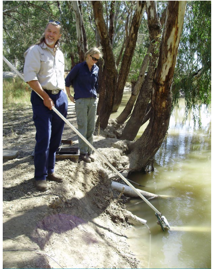
Danny Hannon and Sophie Gatacre of the New South Wales Office of Water deploy a SonTek-IQ shallow water flow meter in Colombo Creek, part of the Murray-Darling river system.
