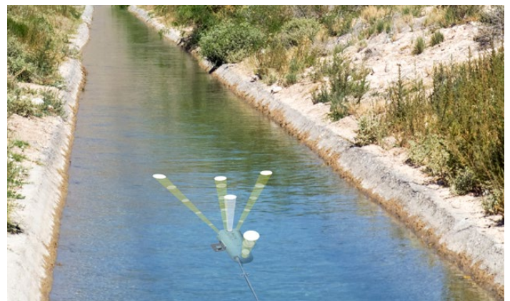
The SonTek-IQ is a Doppler current meter designed for water velocity, level, and flow measurements in the field. The IQ provides the technological advantages of complex/expensive current profilers, but in a simple, inexpensive, and easy to use package.
