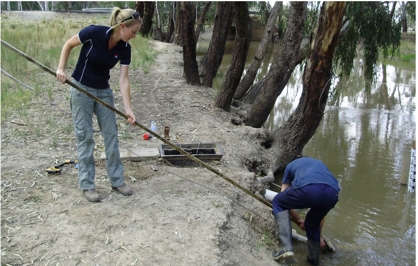
Hydrographers Sophie Gatacre and Simon Turner of the NSW Office of Water adjust the platform under a SonTek-IQ shallow water flow meter, preparing for accurate flow and level measurements in slow-flowing Colombo Creek.
